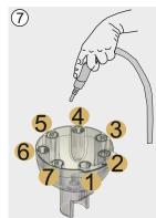
**8.** Remove the ultrasound from the parking position (without the working tip on) and position the handpiece in the CleanHub (position 3-7).
