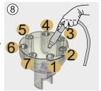
**9.** Take the multifunctional syringe(s) out of the parking position (without cannula attached) and position it in the CleanHub (position 1-2).
