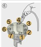
7. Take turbine connection with attached Unifix (multiflex coupling) out of the parking position (without attached transmission instrument) and position it in the CleanHub. Ensure that the water regulation on the Unifix (multiflex coupling) is open. (position 3-7)
