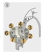
**10.** Take the suction hose (OP suction or saliva ejector) out of the park position and put it on the suction nozzle to suck off residual water.
